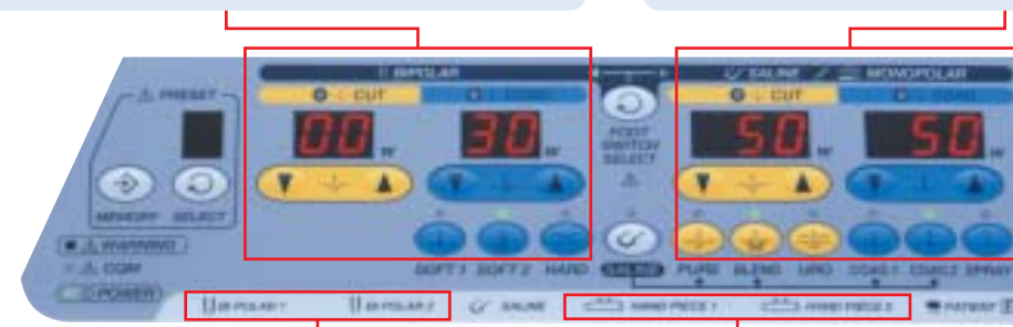
Two Separate Connectors for Monopolar and Bipolar
